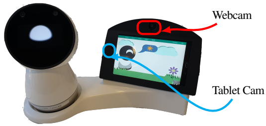
Fig. 1: A portable station that integrates a social robot, a tablet, and a Raspberry Pi with a wide-angle USB camera.
