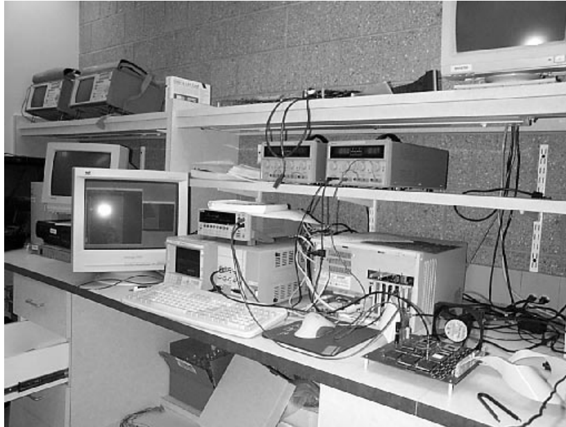
Figure 5.45: DCT Chip Test Setup Photograph
