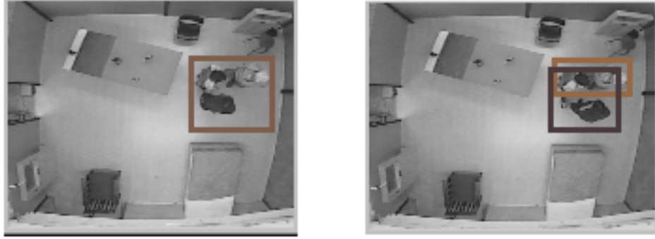
Figure 3-5: Segmentation when people are close to each other: The left picture shows a merge where people are lumped into one blob. The right picture shows unreliable segmentation due to proximity. The squares shown are the bounding boxes of the blobs found in the image.
