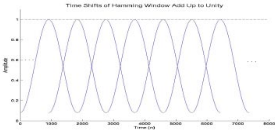
Figure 5.7. Shifted copies of the window w[n] add up to unity (dashed line).
