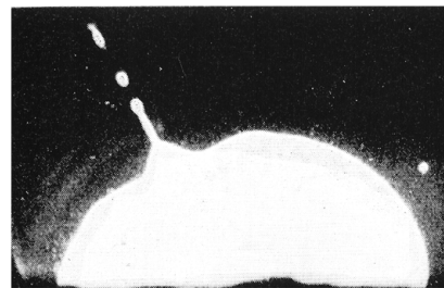
Figure 3.12 How spatter can form from liquids when gas bubbles escape (Richardson, 1974) (a) series of events in the bursting of an air bubble about 0.5 cm across on the surface of water (b) ejection following burst of 50 mm 3 bubble of N 2 from 1.0 cm mercury drop (c) ejection caused by bubble of CO bursting from carbon iron drop about 0.8 cm across, levitated in flowing oxygen Reprinted with permission from Elsevier.
