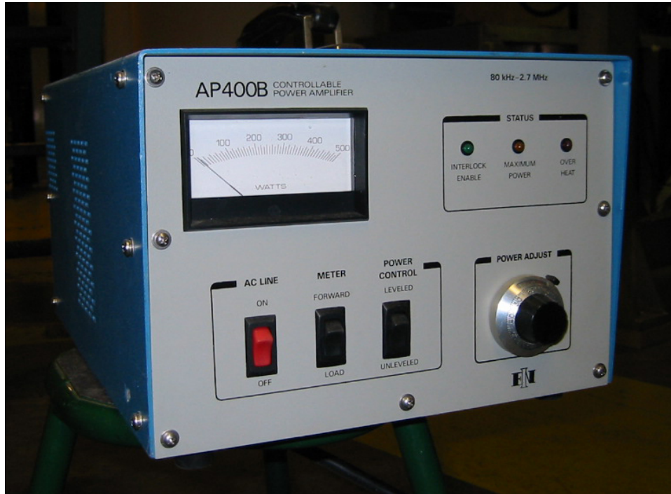
Figure 3-14: ENI AP400B commercial amplifier, capable of delivering 400 W into a 50 \Omega matched load
