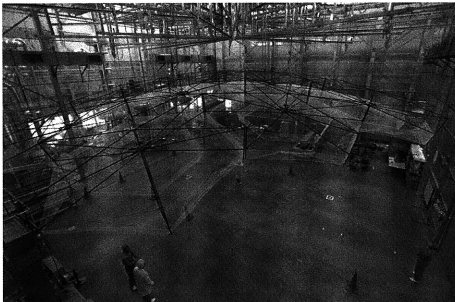
Figure 3-6: LDR engineering model deployment test (Copyright: NASDA)
