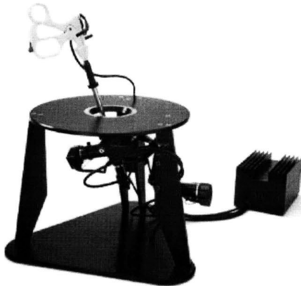
Figure 2-5 Virtual Laparoscopic Impulse Engine by Immersion Cooperation
