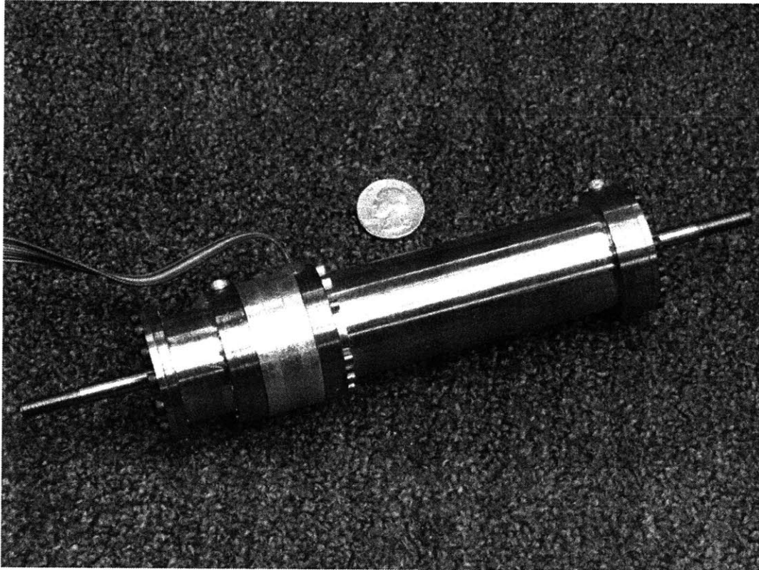
Figure 8.1 Photo of sealed, self-contained electro-hydraulic actuator
