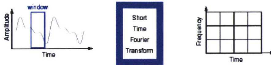
Figure 3-5: Visual representation of the process of making STFTs
