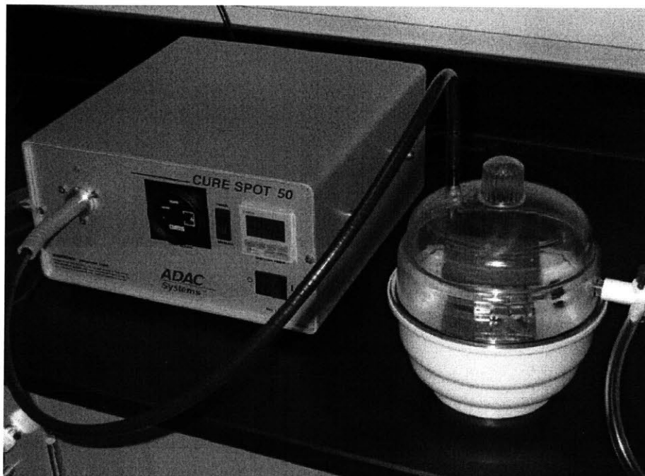
Figure 17: Nitrogen Purging Chamber Coupling with UV fiber
