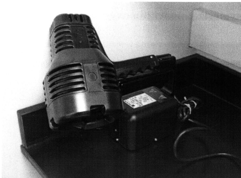
Figure 18: UV lamp with 10\text{mW}/\text{cm}^2 intensity
