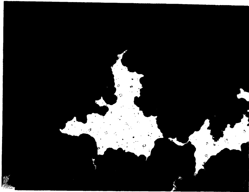
Figure 4.1.10. b) Photograph (x100) of a region of the coating after the 100-day exposure. The light islands (Al) represent adhered areas. The surrounding black areas (Al(OH) 3 ) represent delamination.
