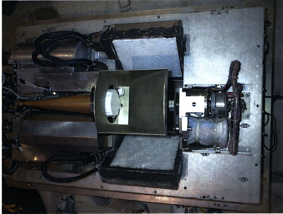
Figure 3-6: Top view of NAST-M horns, reflector, and onboard calibration loads
