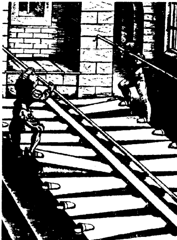
Air pump for the Halberstadt organ in the 16th century (from Praetorius).
