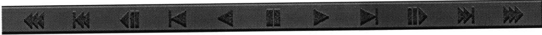
Figure 75. The eleven Movie Controls. From left to right, they are: Scan Reverse, Jump Reverse, Frame Reverse, Reverse Play Extent, Reverse Play, Pause, Play, Play Extent, Frame Forward, Jump Forward, and Scan Forward.
