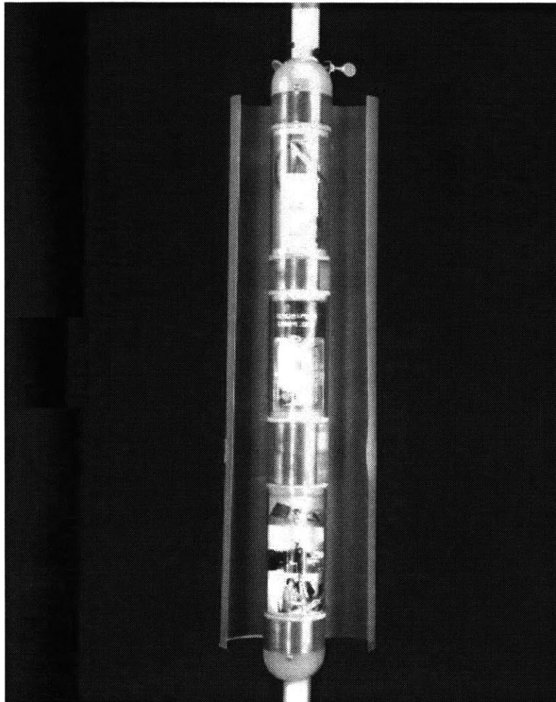
Figure 7-11: The body of the field sensing staff, with the doors open. The relic containers are bracketed above and below by field sensing electrodes.
