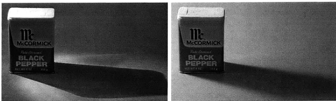
Figure 1-12: Photographs of shadows due to small and large area light sources. (Left) The box of pepper is illuminated by a small flashlight, which leads to sharp shadows. (Right) The box is illuminated using a large desk lamp, which leads to softer shadows.
