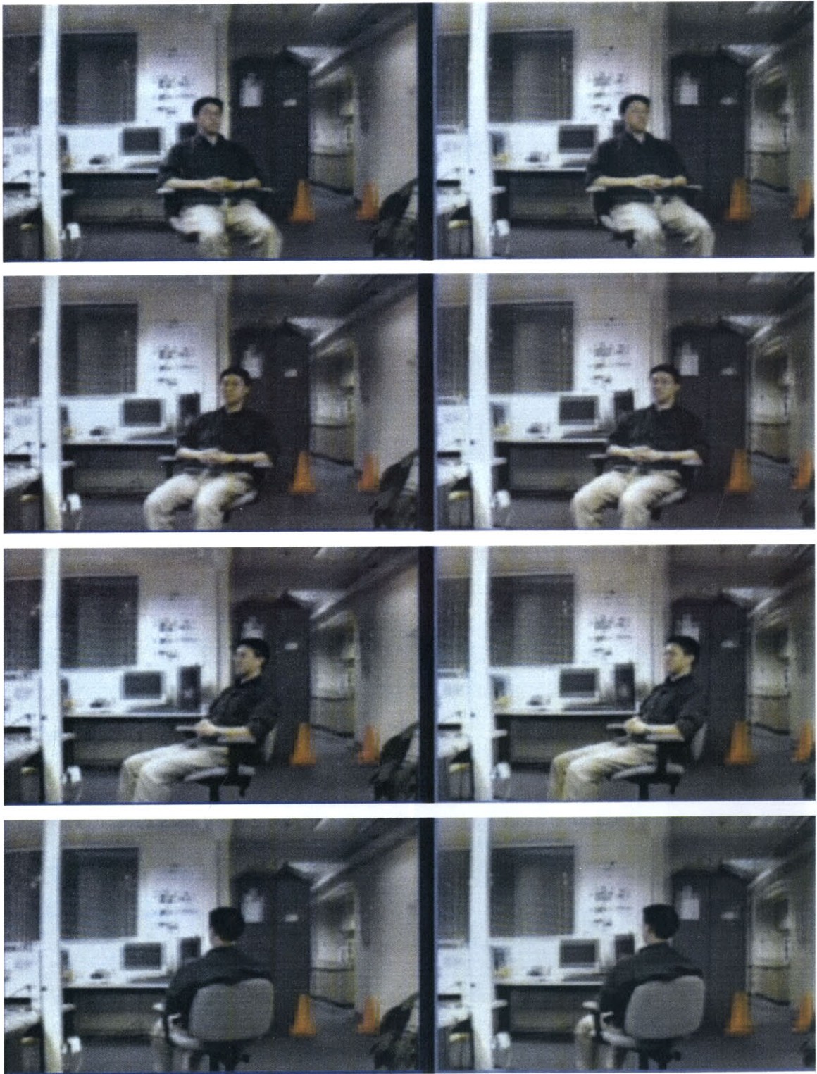
Figure 7-5: Stereo Images. Sequence of stereo pairs from a video capture from the prototype camera array. 3D viewing is possible by cross-eyed fusing each image pair.
