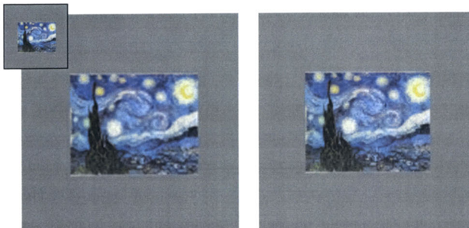
Figure 5-19: Enlarging an exactly sampled image (left) vs. rendering at a high resolution (right). Although the images are not exact, the effect is still a blurry image.
