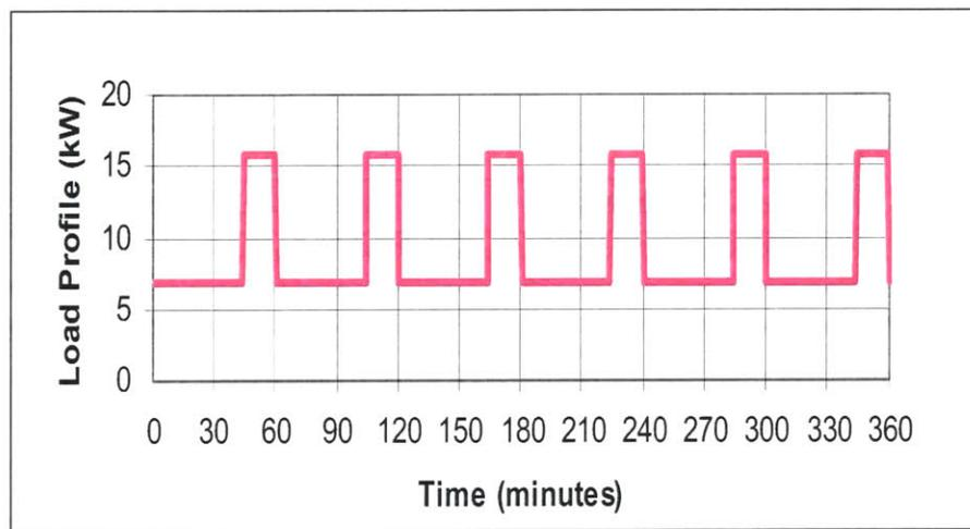
Figure 3.1 Load Profile Model for former NEXTEL Base Station, Cross St., Cambridge, MA
