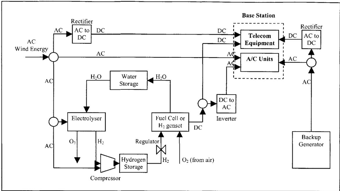
**Figure 2.1 Components, Energy and Mass Flows of proposed Wind-Hydrogen Power Supply System**
