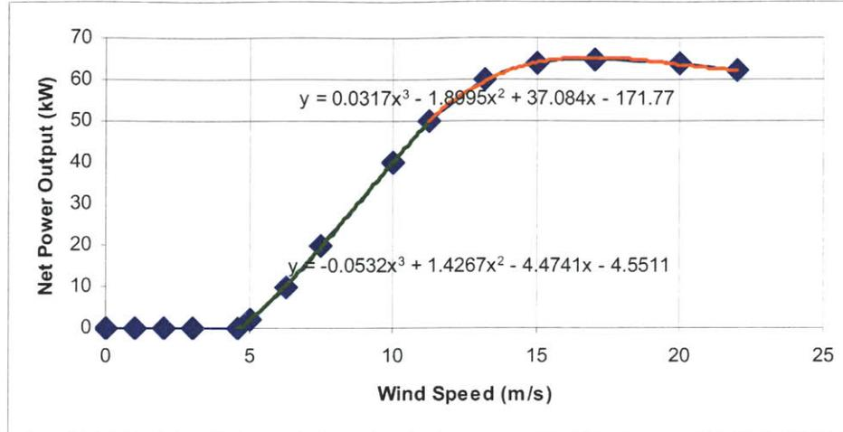
Figure 3.2 Power Curve & Polynomial Functions for the Wind Turbine Model
