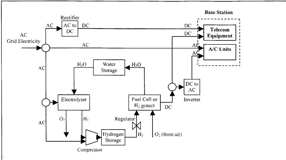
**Figure 2.3 Components, Energy and Mass Flows of proposed Peak-Shaving Hydrogen Power Supply System**
