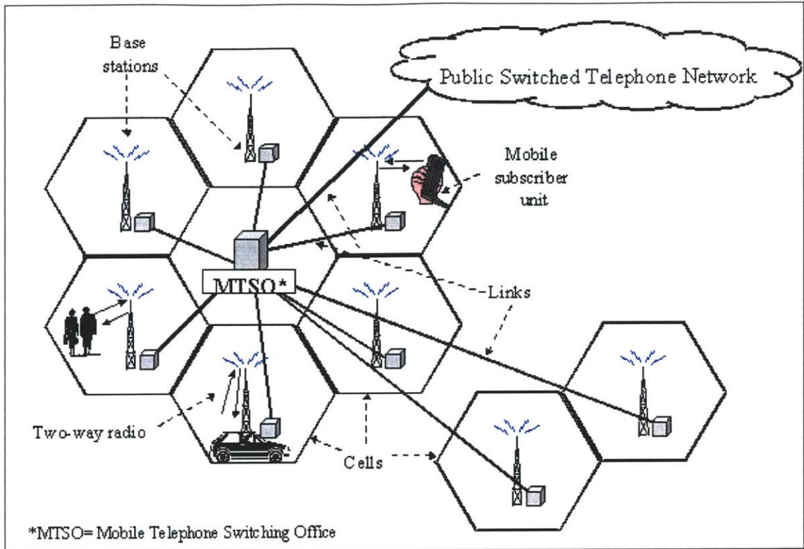
Figure 1.1 Schematic of the Cellular Telephone Network\*
