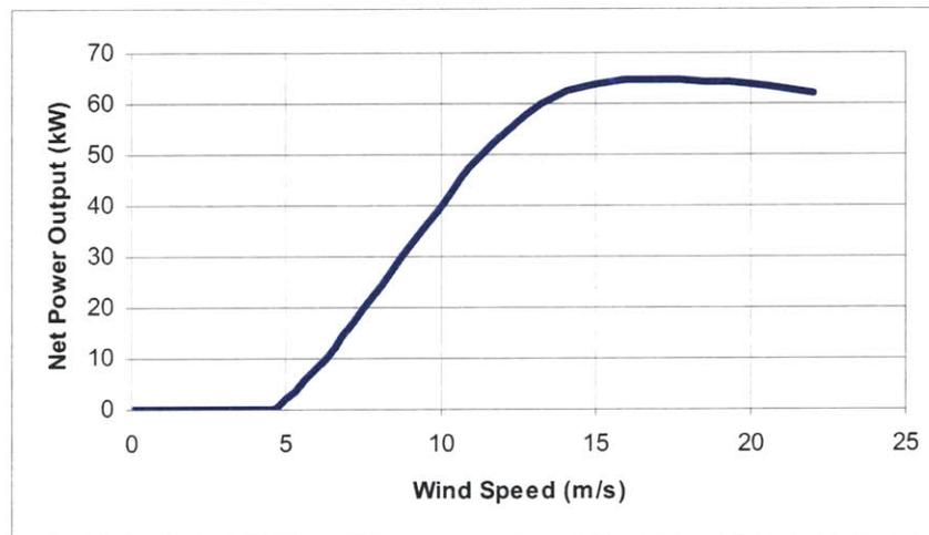
**Figure 2.2 Power Curve of an AOC 15/50 50kW Wind Turbine**
