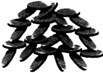
Figure 2: A three dimensional structural form of Laponite which shows the electrostatic attraction forces on the faces and edges of the surrounding Laponite crystals [7].
