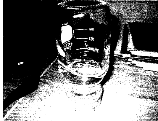
Figure 12: A sample of 3% wt. Laponite solution, upside down after being shaken, showing the viscous fluid-like properties.
