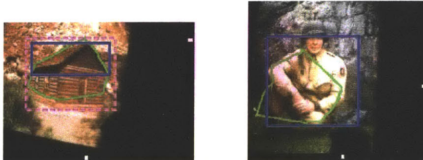
Figure 10. Interesting failure modes for Experiment 3. At left, the eyetrace intended to capture the cabin instead captured its roof, a much stronger color region. The natural image at right illustrates a problem inherent to color-based object segmentation; the algorithm has no notion that the soldier's white face and gray helmet are both part of the same object. It may be possible to address this issue with a region unification algorithm.
