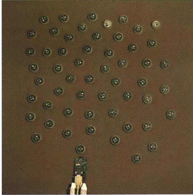
Figure 2-3: The 1.2-m by 1.2-m substrate into which the Pushpins are pressed provides a power and ground connection for the nodes, alleviating the need for batteries. The gateway node at the bottom of the image provides two-way communication between the network and a PC.
