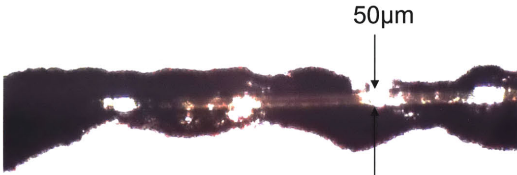
Figure 17 Optical microscope image of non-uniform polypyrrole coverage from chemical deposition on hollow microfiber.
