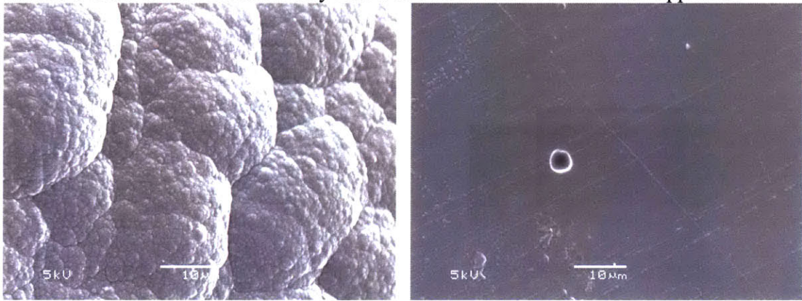
Figure 5 Bumpy and smooth morphologies of electropolymerized polypyrrole films. Low temperature polymerizations ( -40 to -20^\circ\text{C} ) produce high conductivity films ( 10^4 S/m) with smooth surface morphology.
