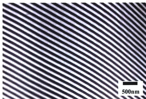
Figure 31 Transmission Electron Microscope (TEM) image of lamellar morphology for PS-PI. Domain spacing: 100 nm. Sample cast from toluene solution, thin sliced with a microtome. PI block stained with osmium tetroxide ( \text{OsO}_4 )
