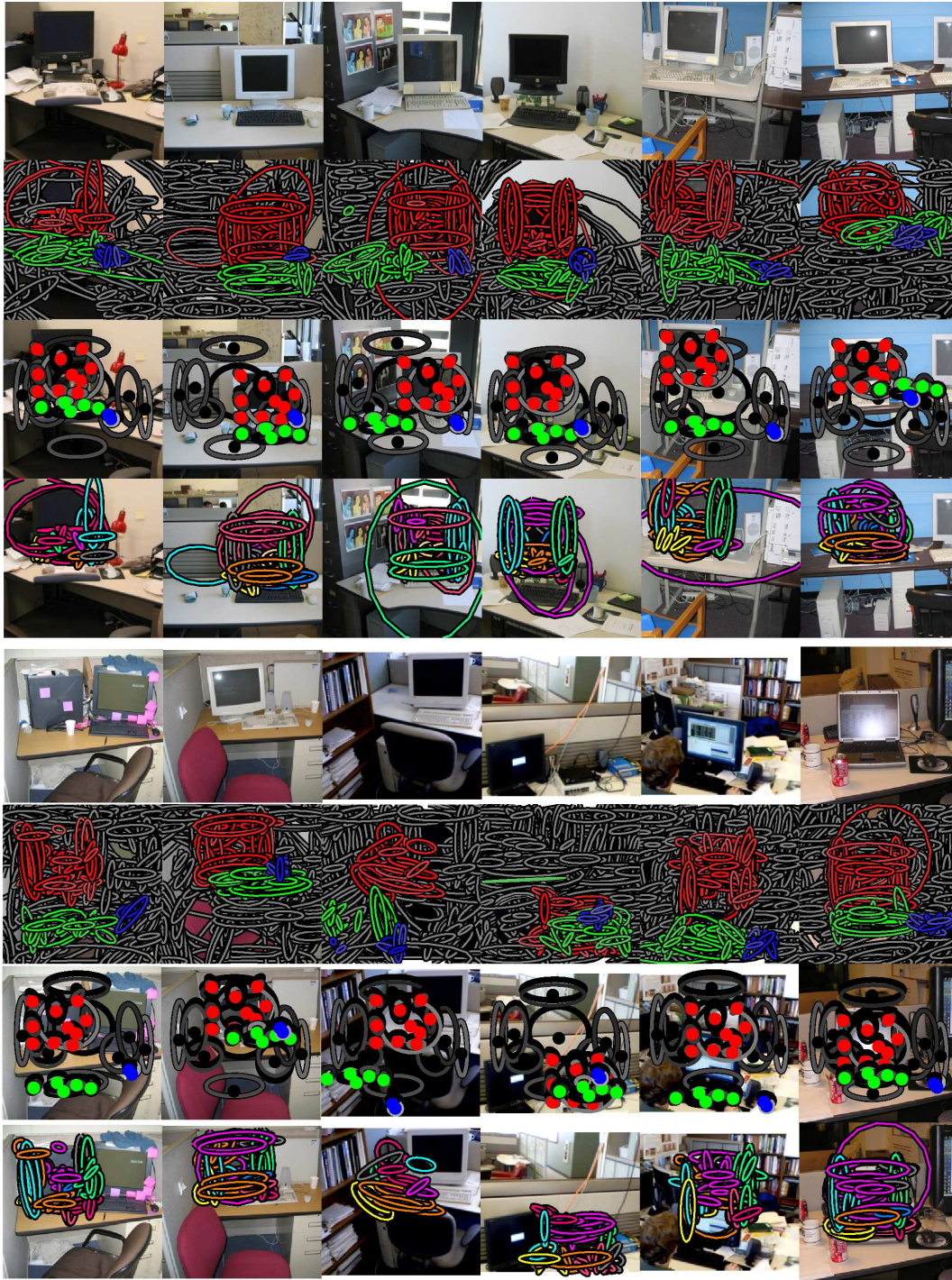
Figure 6.6. Feature segmentations produced by a contextual, fixed-order model of office scenes containing computer screens (red), keyboards (green), mice (blue), and background clutter (gray). Each block of four rows depicts six test images (first row). Feature segmentations (second row) assign each feature to the object category with the highest posterior probability. We also show model parts translated according to each image's reference transformation (third row), and color-coded assignments of features to the different parts associated with computer screens (fourth row).
