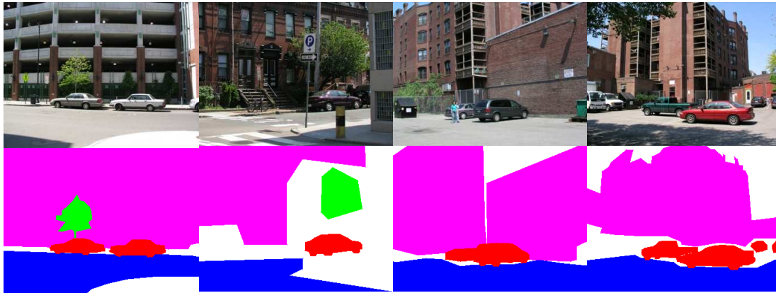
Figure 1.2. Partial segmentations of street scenes highlighting four different object categories: cars (red), buildings (magenta), roads (blue), and trees (green).
