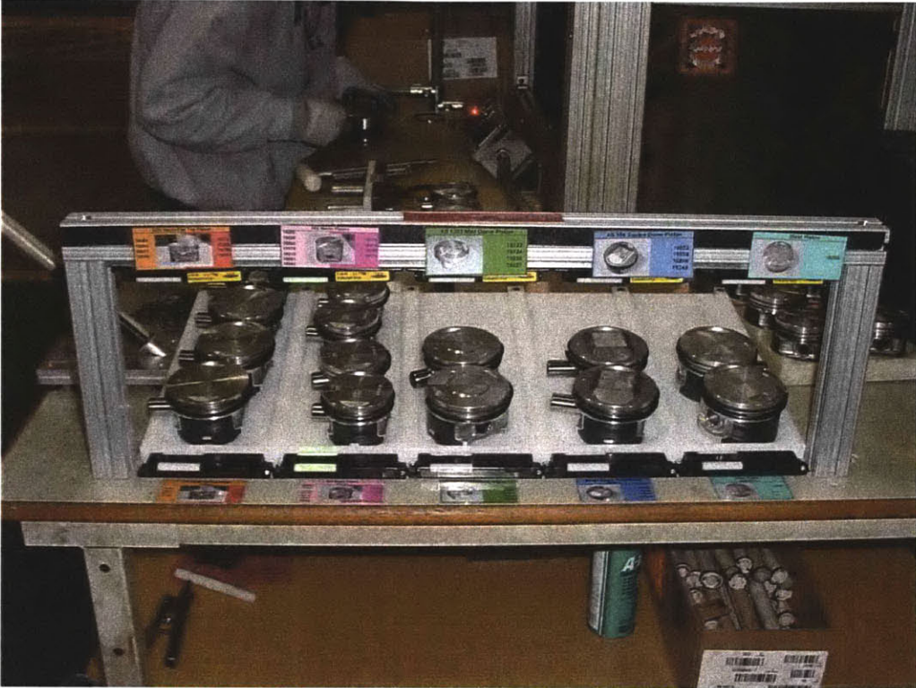
Figure 34: Piston Pick to Light System
