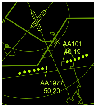
Figure 4.10: Example TRACON ATC scenario in which the lateral separation state is progressively reducing.
