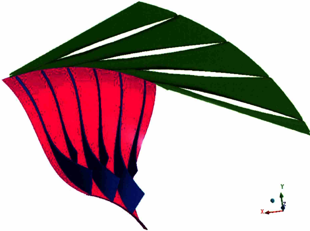
Figure 2-5 Domain used in 3D unsteady model which includes 3 impeller passages and 4 diffuser passages
