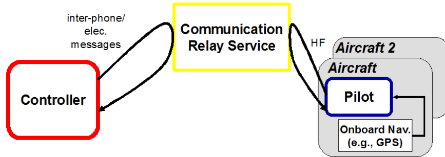
Figure 2-1: Current Controller-Centered Control Loop for oceanic ATC. Communication is conducted over HF radio through a third party communication relay service. Surveillance is conducted by pilot position reports, which are reported approximately every hour.
