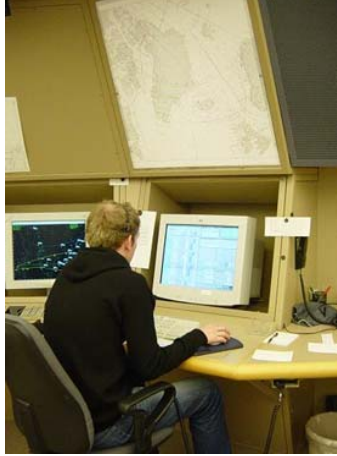
Figure 3-5: The Reykjavik controller workstation consists of electronic flight strips, in front of the controller and a situation display, to the left of the controller.
