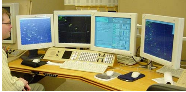
Figure 3-8: Reykjavik Center workstation in a sector with limited radar coverage. The screen on the left is the situation display. The second screen from the left and the screen on the far right display radar information, two screens are provided so that the controller can see an overview of the traffic and zoom in on a conflict at the same time.
