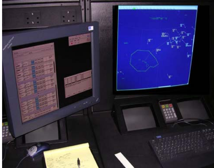
Figure 3-14: ATOP is the future oceanic ATC workstation scheduled to replace ODAPS in the U.S. facilities in 2004 and 2005.
