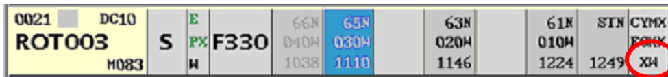
Figure 3-7: Equipment information is located on the flight strip. This aircraft is equipped for MNPS (“X”) and RVSM (“W”).
