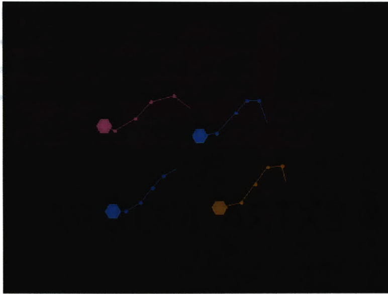
Figure 5-3: Faulty data aggregation, due to inadequacies in the data association function, leads to multiple aggregates created for a single object, which leads to multiple cursors for the same ball. SensorDataStrands in the same SensorDataAggregate are represented by hexagons of the same hue.
