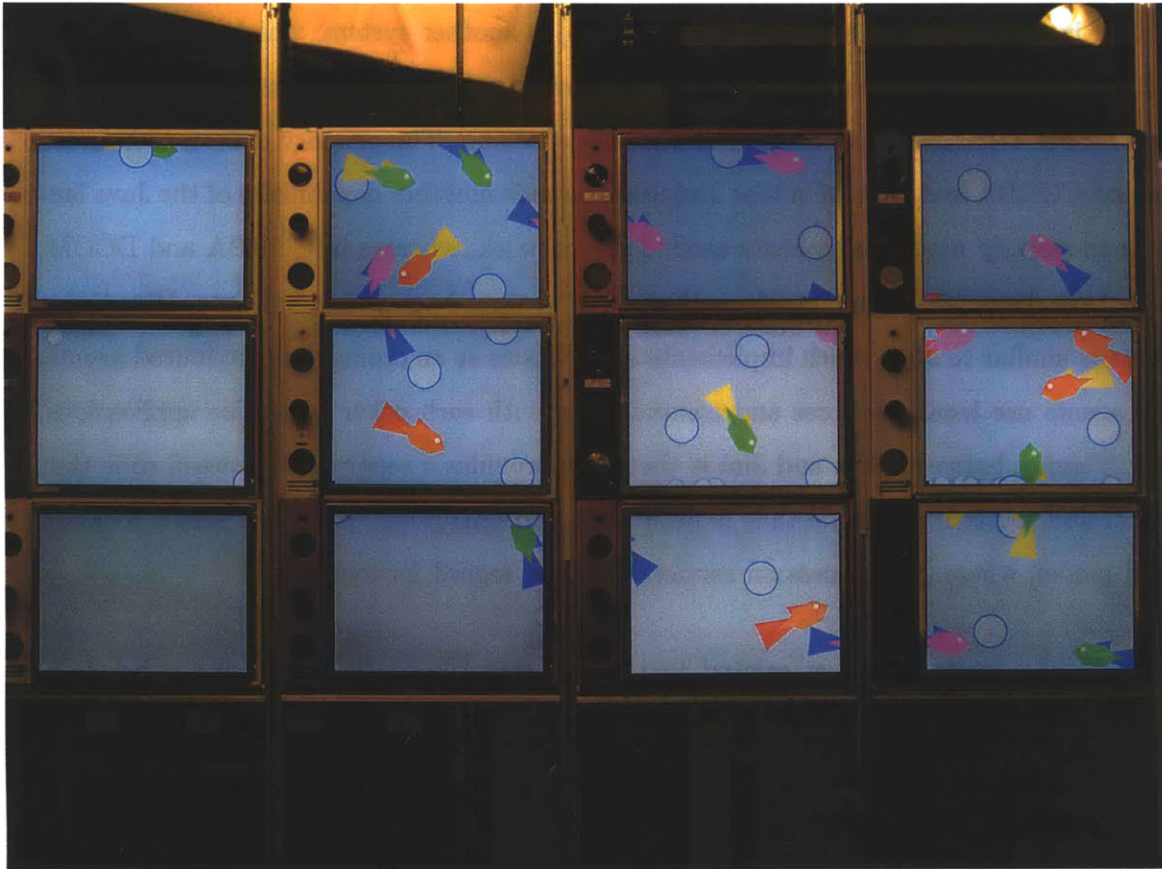
Figure 1-1: The tiles are shown running the distributed simulation. There are a number of instances where pieces of different agents appear across multiple tiles.
