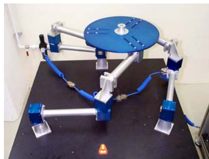
Figure 12: 3-DOF planar modular parallel robot
