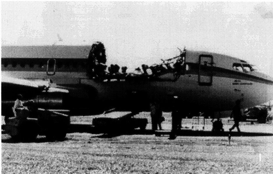
Figure 2.1: An aircraft damaged due to corrosion [4].
