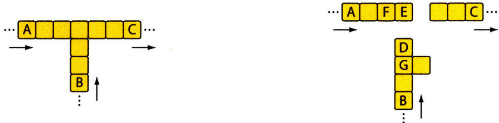
(a) OR gadget. If the tipper can reach either A or B, then it can reach C.
