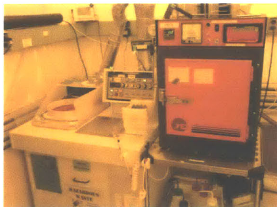
Figure 4.11- (Right) HMDS vacuum oven, (left) Photoresist spin coater
