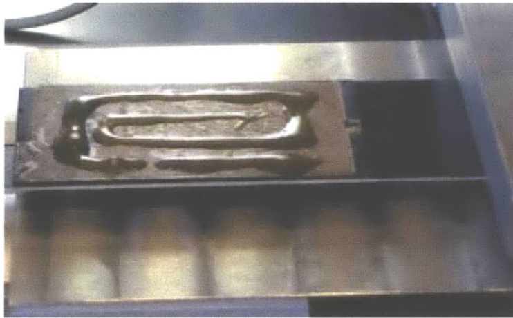
Figure 5.13- ER fluid was injected onto the chip (subsequently spread with a spatula/squeegee)
