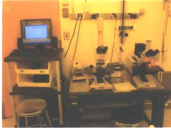
Figure 4.14- Nikon inspection/measuring microscope and fluoroscope
