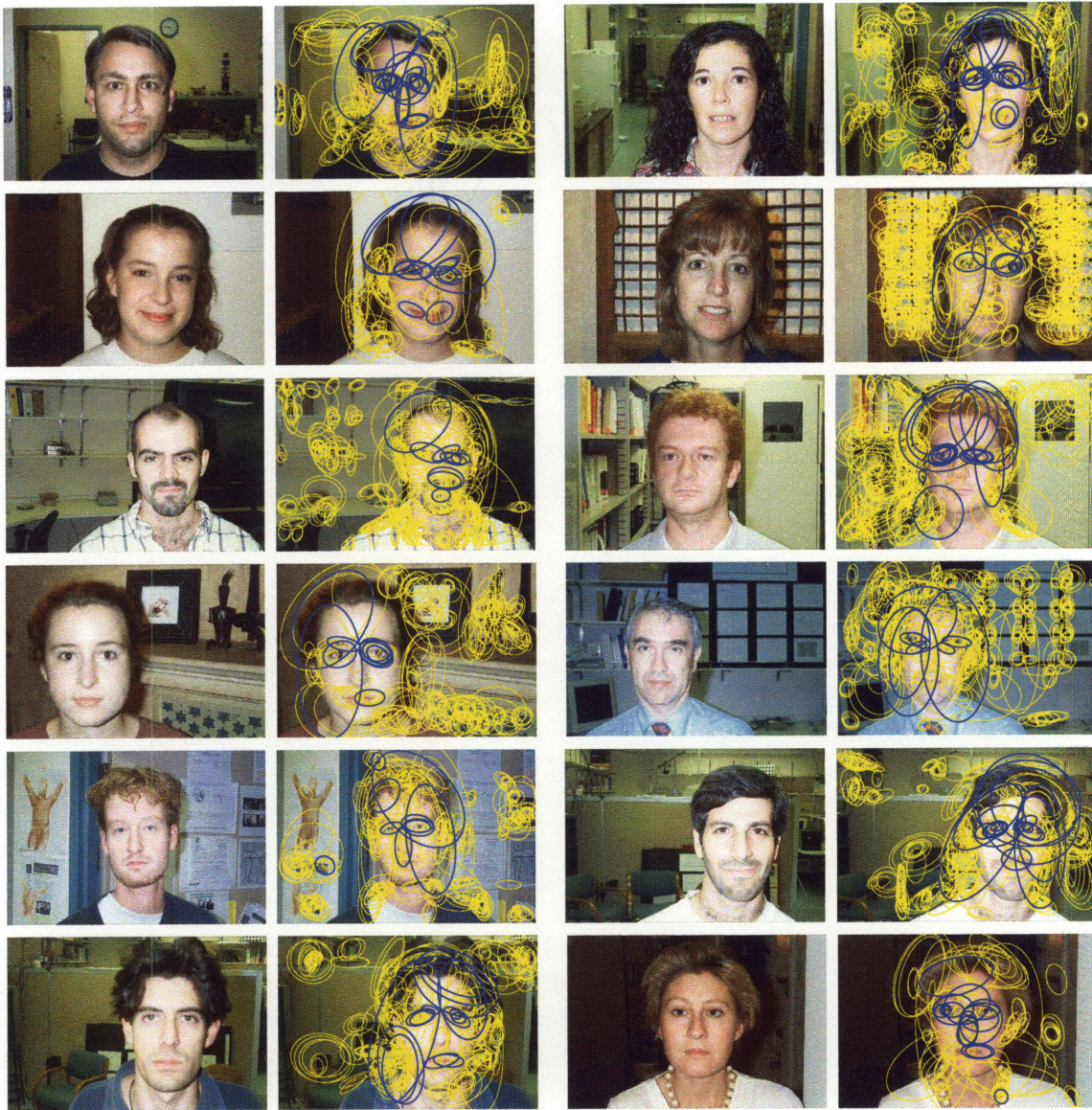
Figure 9-4: Inferred feature masks for a face category. The elliptical regions indicate where features were extracted from the images based on the Harris-Affine interest operator. The boundaries of these regions are color-coded in order to show which features contribute most strongly to each image's matchings against the other face images: blue (darker colored) ellipses denote the features in each image with the high weights in the mask, and yellow (light colored) ellipses denote the remaining features, which have low weights in the mask. Each entry in an inferred feature mask reflects how consistently that feature can be matched against all other images in a cluster. These examples demonstrate how the inferred feature masks reveal which parts of the images correspond to the in-class category, and can be used to downplay the impact of background or clutter features in the matching. (This figure is best viewed in color.)
