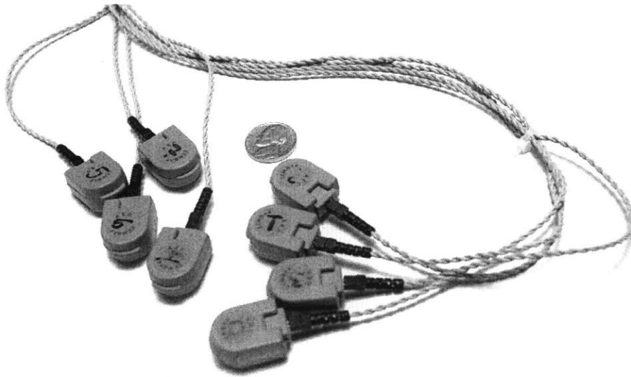
Figure 3-2: The 8 tactaid actuators used in this initial experiment.
