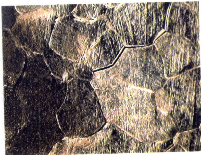
Figure 7.2.12. Surface discontinuity at crater of TT-2
