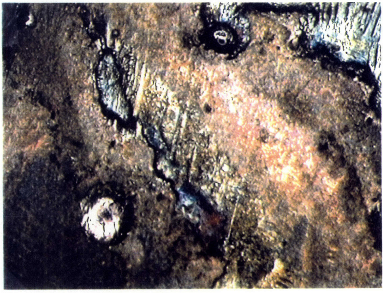
Figure 7.2.5. Surface discontinuity at crater of ST-3
