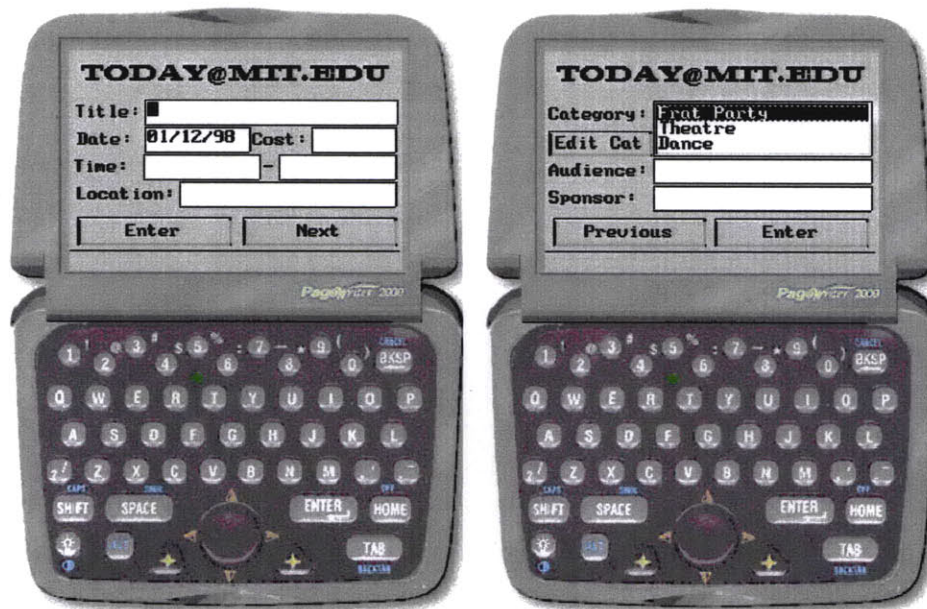
Figure 4-24: The freshmen designed a pager interface with which to submit campus events to a calendar database server.
