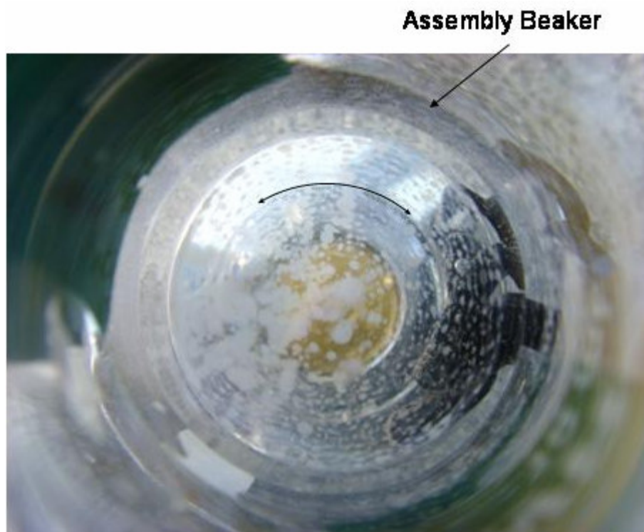
Figure 6. 10 Top view of an aggregation pattern of microspheres at the bottom surface of the assembly beaker during ultrasound excitation. A curved arrow is drawn to highlight the concentric pattern of the aggregation at the peripheral region of the bottom surface. The pitch between the rings is 0.8 mm. The image of the yellow circular part transmitted through the beaker glass indicates the vibration pad emanating the ultrasound wave into the beaker. The input voltage was set to 55 volts.
