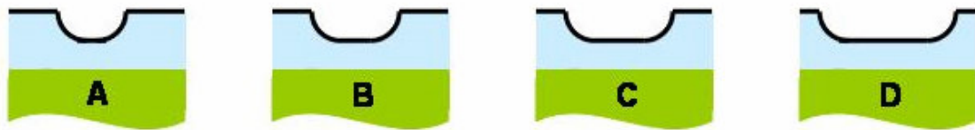
Figure 4. 1 Pattern layout includes 20 arrays, identical, but with increasing exposure dose to form increasingly large holes; close-up of an array showing repeated pattern of four hole shapes (A, B, C, D) corresponding to four different-sized exposure regions. Schematics of four hole shapes (A, B, C, D) after etching are displayed at the bottom.
