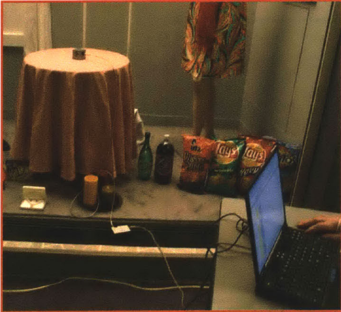
Figure 35 – Procedure to measure the light spectra from incandescent and LED lighting systems were conducted at Osram-Sylvania Lighting Research Center and used an spectroradiometer with operation and data reduction by OSRAM SYLVANIA proprietary software.
