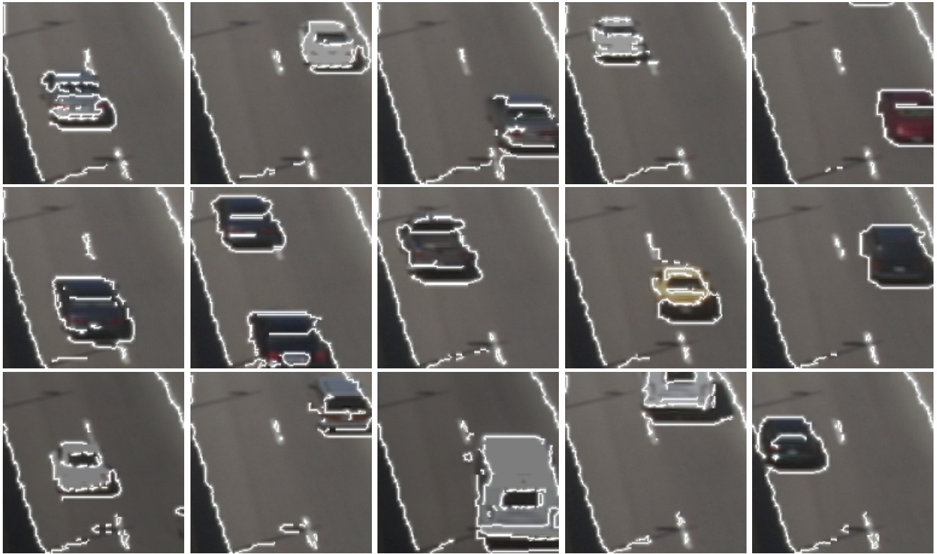
Fig. 6. These results were inferred by the car model on images drawn from another road's traffic. The results required 40 candidates per node and 20 iterations of belief propagation. The model does a good job of extracting the car boundaries, except where the car colors blend into the road too much, or where there is competition between car contours and strong road contours.
