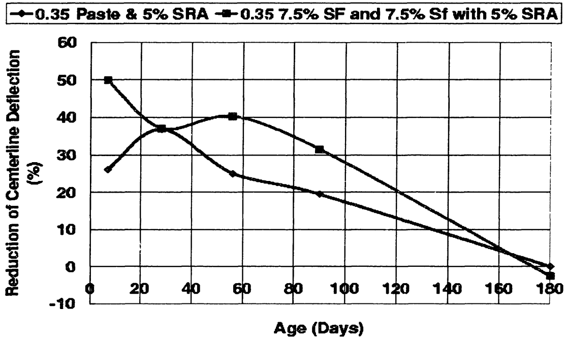
Figure 4.3.6 The reductions in curling deformations experienced by the W/C = 0.35 mixes.
