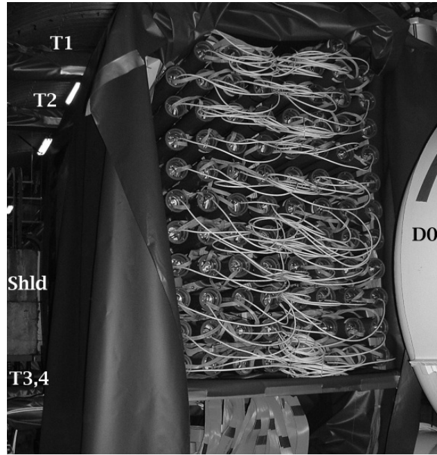
Figure 2.12: A photograph of the fully commissioned Au-PCAL. Easily seen are the PMT mountings and readout cables. To guide the eye, certain features have been labeled: the cosmic ray trigger modules (T1-T4), the shielding (Shld) and the D0-magnet (D0). During normal operation, the Kevlar tarp covered the full box, to help prevent light-leaks.
