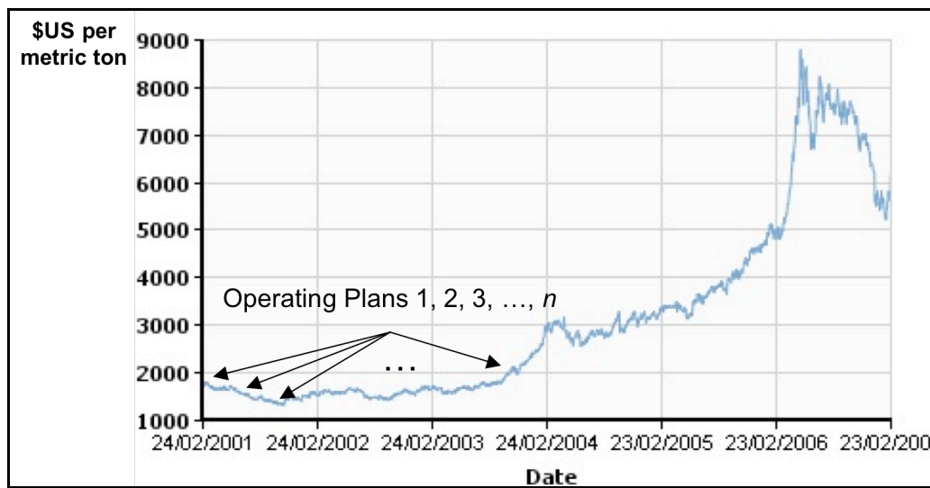
Figure 2.5: Perfectly tailored operating plans represent an upper bound on the highest achievable NPV for a given system. A catalog of operating plans tries to approximate this ideal situation with fewer operating plans.
