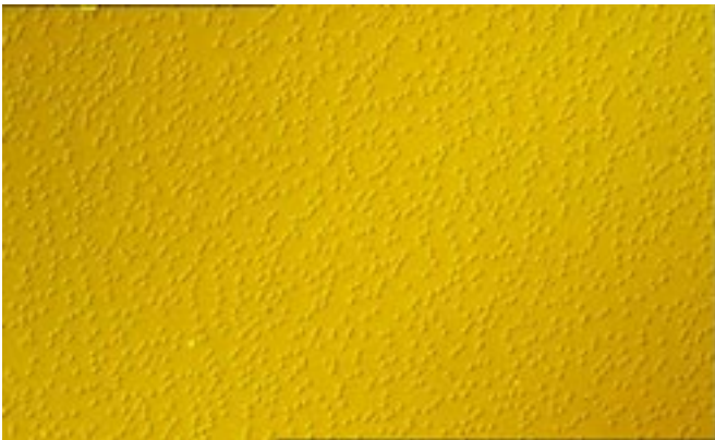
Fig.4: A light microscopic picture of the InGaAsN growth surface.
