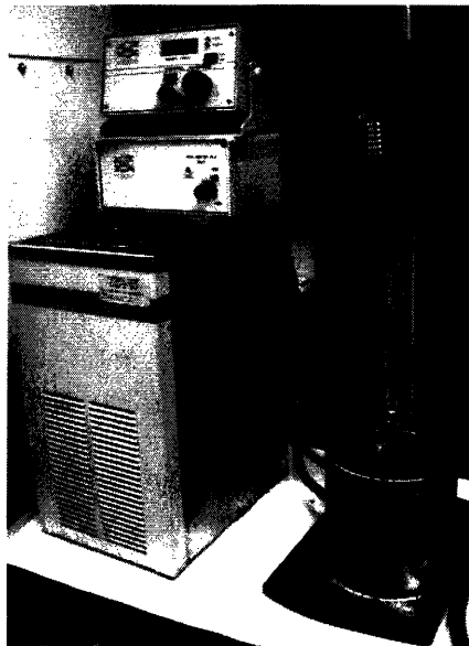
Figure 3.3 Blending apparatus with cooling system attached
