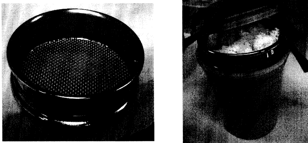
Figure 3.1 1000 \mu m sieve and shaking apparatus used
