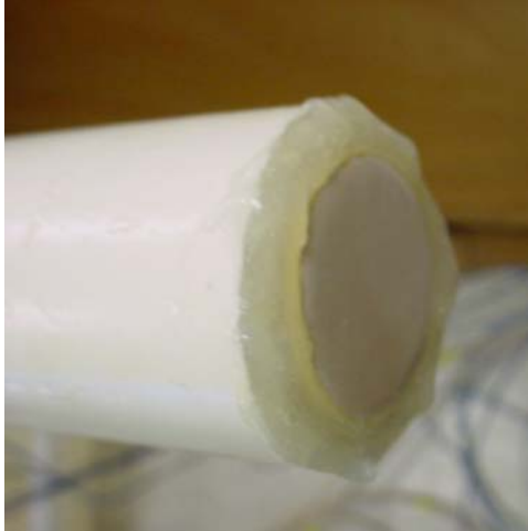
Figure C-5: PVC tube with ceramic cup glued to the end.
