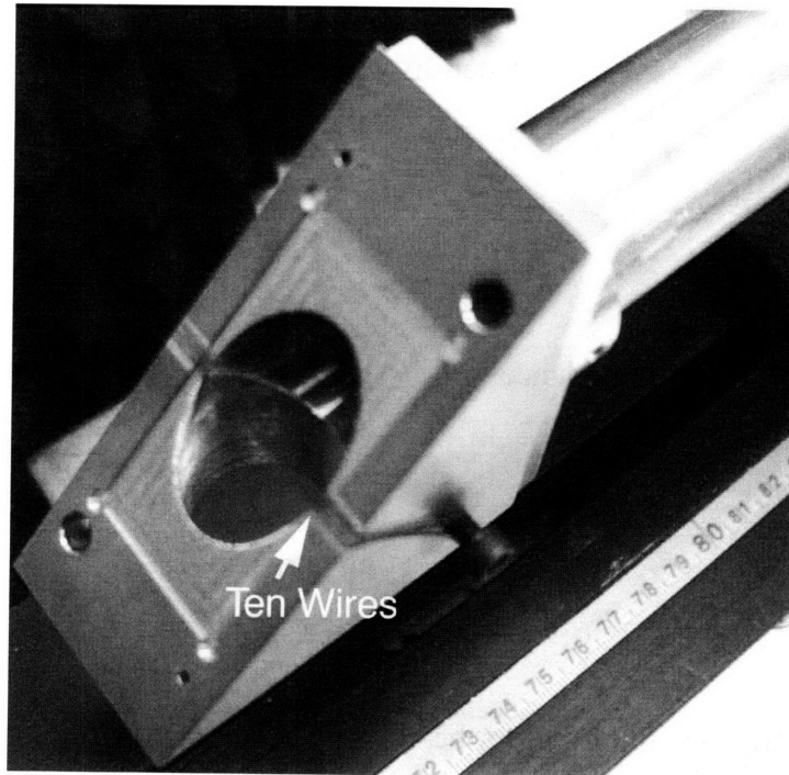
Figure 4-5: View of 10-wire, gauge 36 beamsplitter stretched across the diagonal face of the corrugated 4-port directional coupler block.
