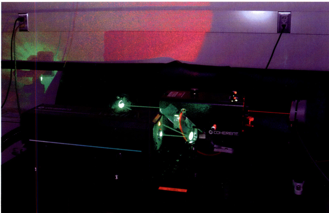
Figure 2-37: System employed for variable-wavelength light irradiation of samples. It consists of a Coherent Verdi DPSS laser (6W, 532 nm) which pumps a Coherent 599 dye laser to produce longer wavelength red light.
