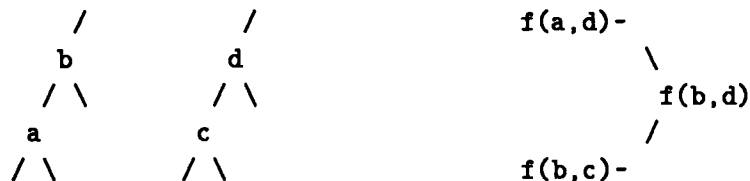
Figure 3. An example of imaging. Suppose that a = b and c = d are true, and that the corresponding equality trees are constructed as shown at the left. The terms f(a, d) and f(b, c) will both have the image f(b, d) , and will therefore both be made equal to f(b, d) .
