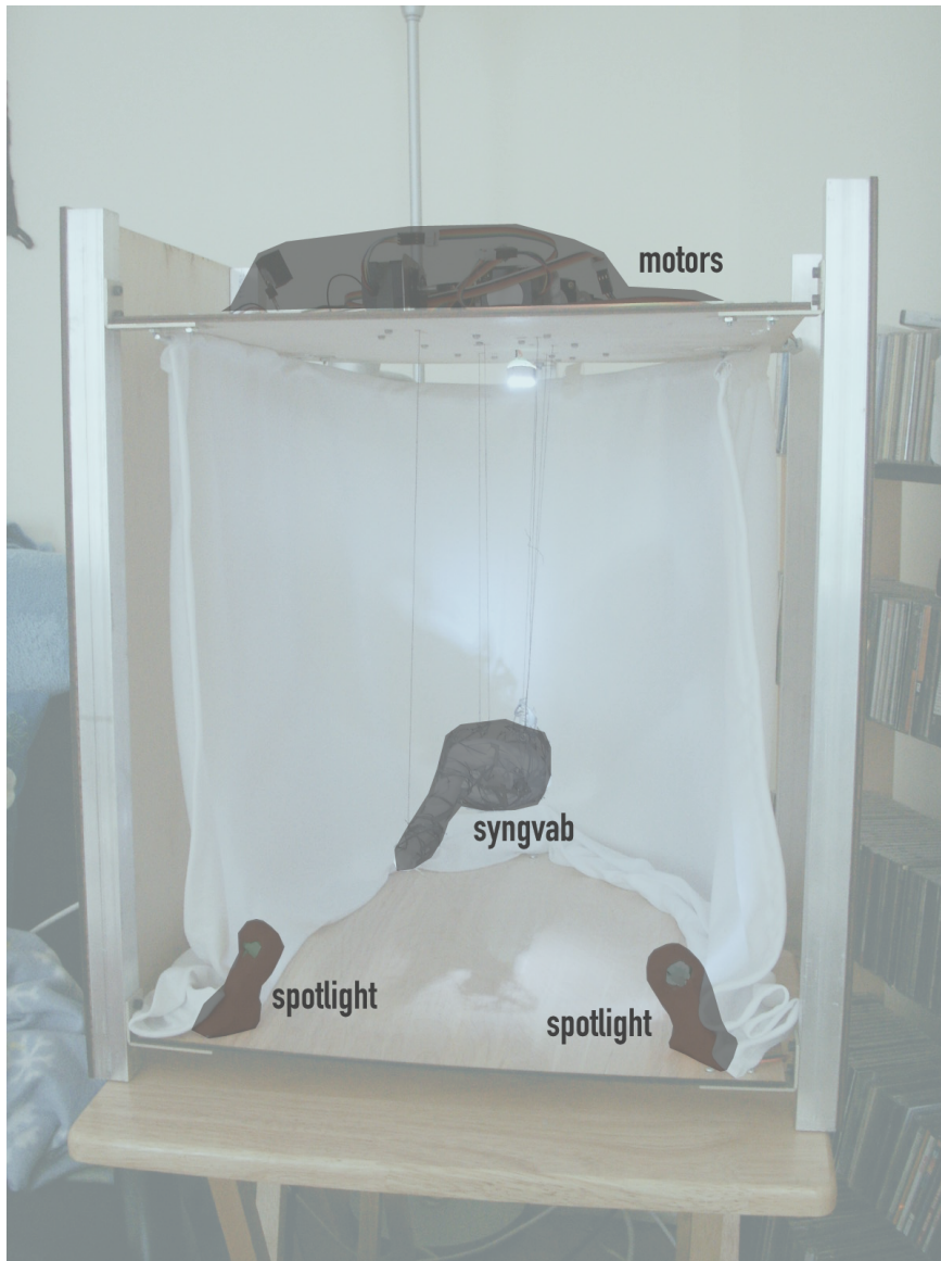
Figure 6.9: Diagram of syngvab , including the creature itself, location of motors, and stage spotlights. A video of the first movements of syngvab can be found at http://purl.oclc.org/NET/NKNOUF/MSThesis/Movies/syngvabFirstVideo.mov , while a video of the final movements with the voice can be found at http://purl.oclc.org/NET/NKNOUF/MSThesis/Movies/syngvabVideo.mov .
