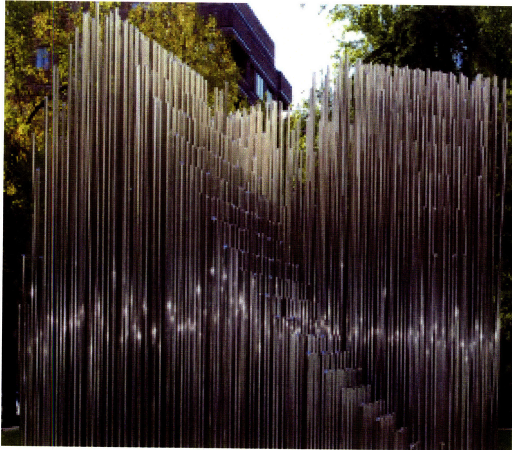
Figure 1.3. Kinematic sculpture by Eusebio Sempere consisting of a periodic array of hollow stainless steel cylinders, each 2.9 cm in diameter, arranged on a 10x10 cm square lattice. This sculpture has been shown to have a partial phononic band gap at 1.67 kHz along the [100] direction [1,22].
